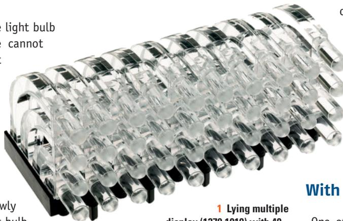
**1** Lying multiple display (1279.1010) with 40 spherical optical outlet faces of 3 mm diameter each; optical outlet face horizontal to PCB; with glare protection
