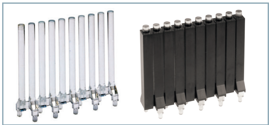
2 Upright multiple display (1272.1020) with ten spherical optical outlet faces of 3 mm diameter each; without glare protection on the left and with glare protection on the right
